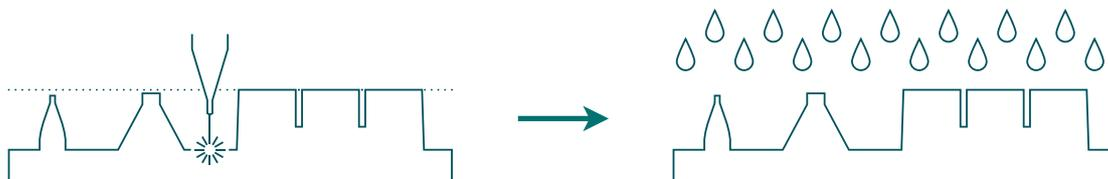
*In direct engraving, the imaging is done in a single step. After subsequent cleaning with a high-pressure water jet and brush, the printing plate is ready for printing.*
