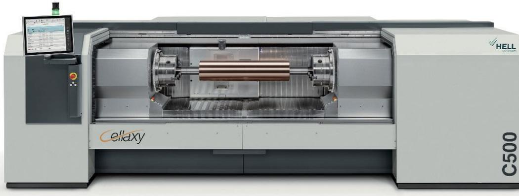
The Cellaxy supports direct laser engraving for linework, contone and embossing rollers.
