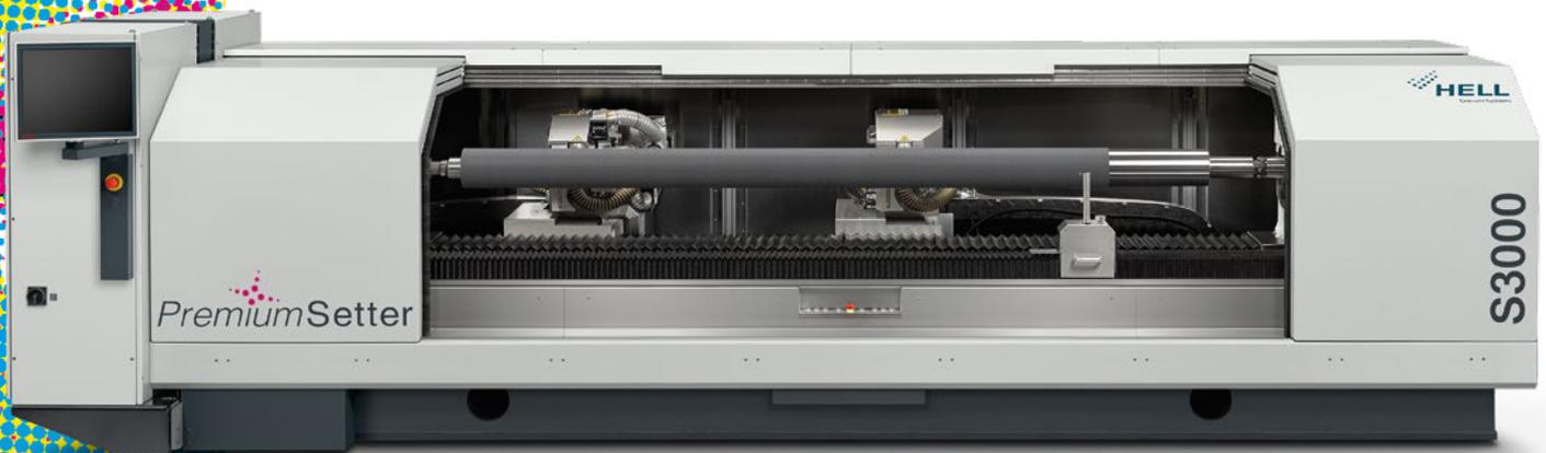
**The PremiumSetter S3000 is an innovative engraving system for direct laser engraving of elastomer flexographic printing sleeves.**
