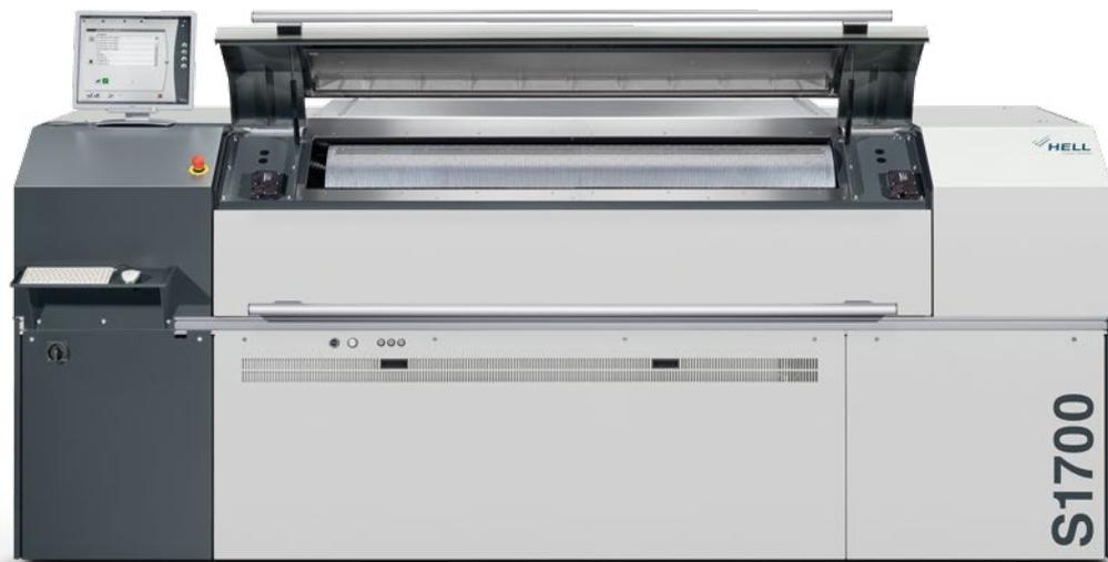
**The PremiumSetter S1700 PL from HELL is an innovative laser engraving system for direct laser-
